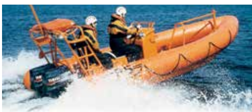
Trelleborg Marine Systems foam fender collar protecting Umoe Schat Harding's R6 fast rescue boat.
