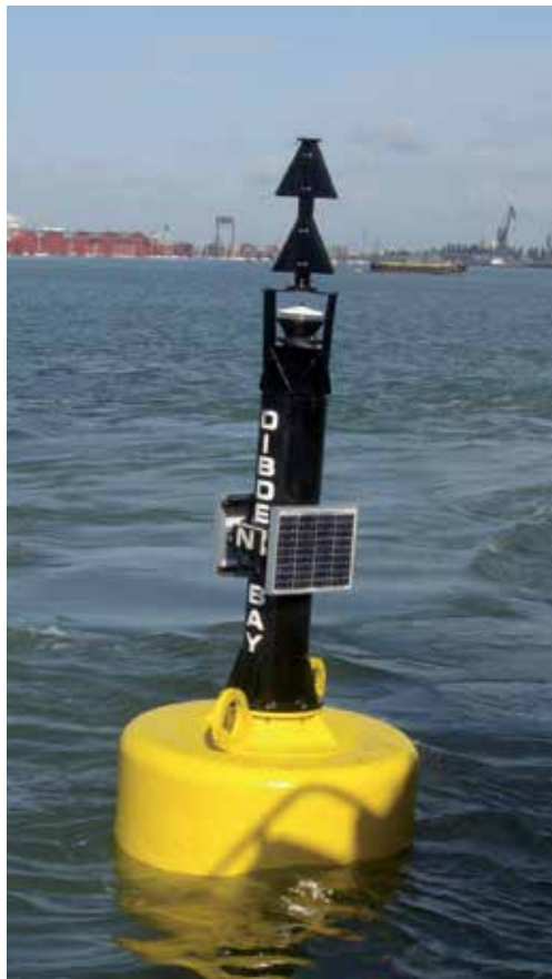
Marker Buoy complete with Daymark and solar powered beacon.
