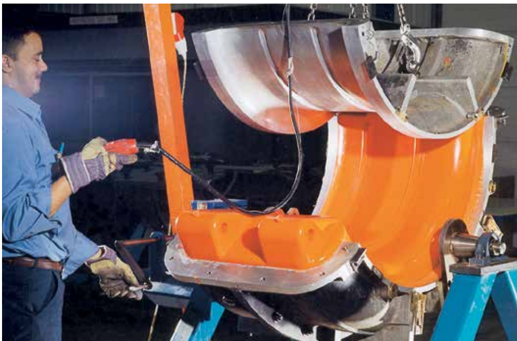
Polyurethane encapsulation of OCIMF hose float.
