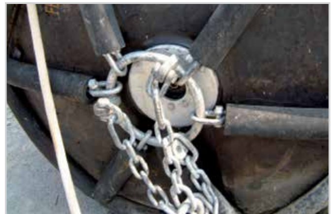
CTN chains connected to the ring shackle on a Type I fender
